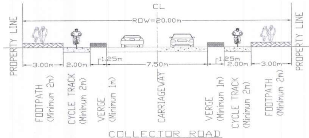
Figure 3: Typical Collector Road Section
